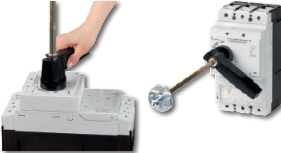
Photo 9: A larger version is necessary to adequately handle the greater forces required to switch the larger frame sizes NZM 3 and 4. An identical „deliberate action“ feature consisting of an initial travel followed by simultaneous pushing and turning motion applies to this handle as well.
