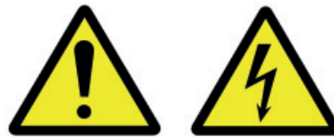
Figure 3: Attention, Dangerous Voltage
