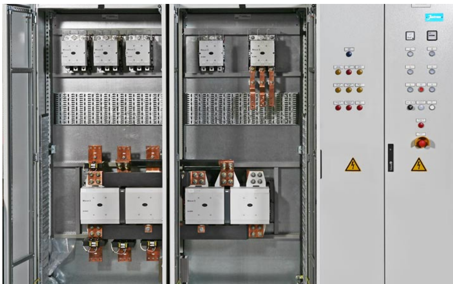
Switchgear for a 700 kW bow thruster system, consisting of two DILM 1600 contactors for controlling the propeller rotation direction and DILM 400/ 300 for the speed control by bridging the resistors in the rotor circuit.
